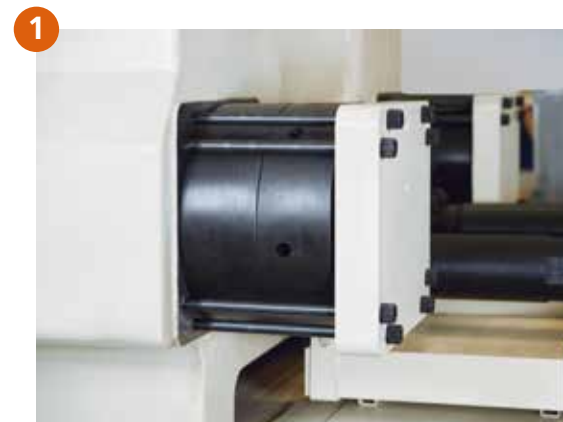
1 Overstress protection mechanism on the nut of the tie bar of the front platen, protecting the tie bar under uneven force.
