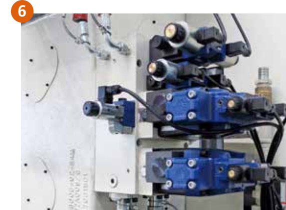
6 Functions such as stable core holding and further push on partial areas to ensure the core holding; automatic pressure relief are available.
