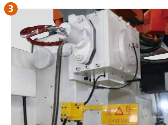
3 Tie bar extraction device available on the upper operation side, and another installation position for such tie bar extraction device is reserved at the back side for option.
